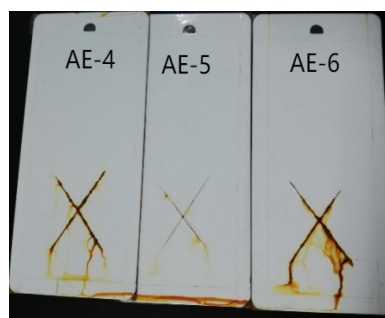
图9 氨基烤漆涂层于盐雾箱中测试144 h后的外观图 Fig. 9 Appearance of Amino Baking Coatings after 144 Hours of Salt Spray Test
