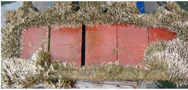
图7 三亚实海挂板试验(防污期效36个月) Fig. 7 The Shallow Water Immersion Test of Sanya (Antifouling Effect for 36 Months)
